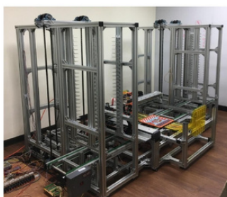
The actual photo for the system of the mosaic tile puzzle machine
